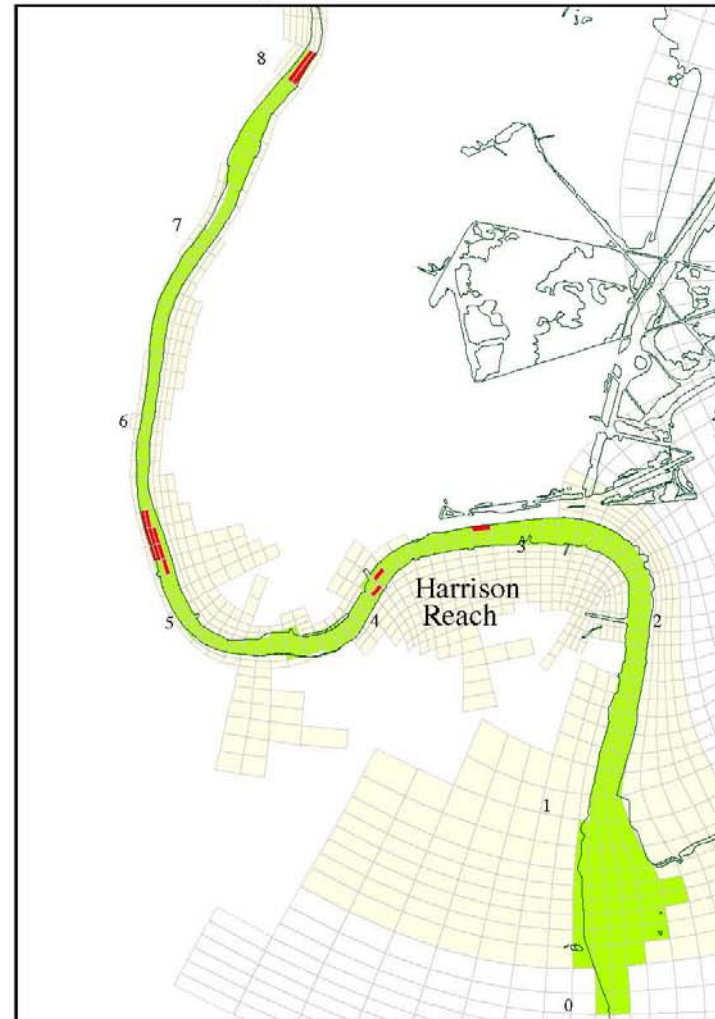
Capping with Dredging for Flooding - Exposed Armor Areas
