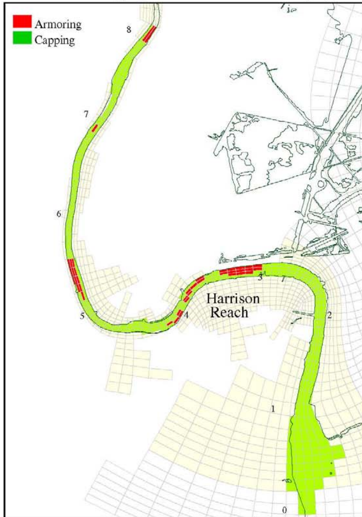
Capping with Armor Area Pre-dredging
