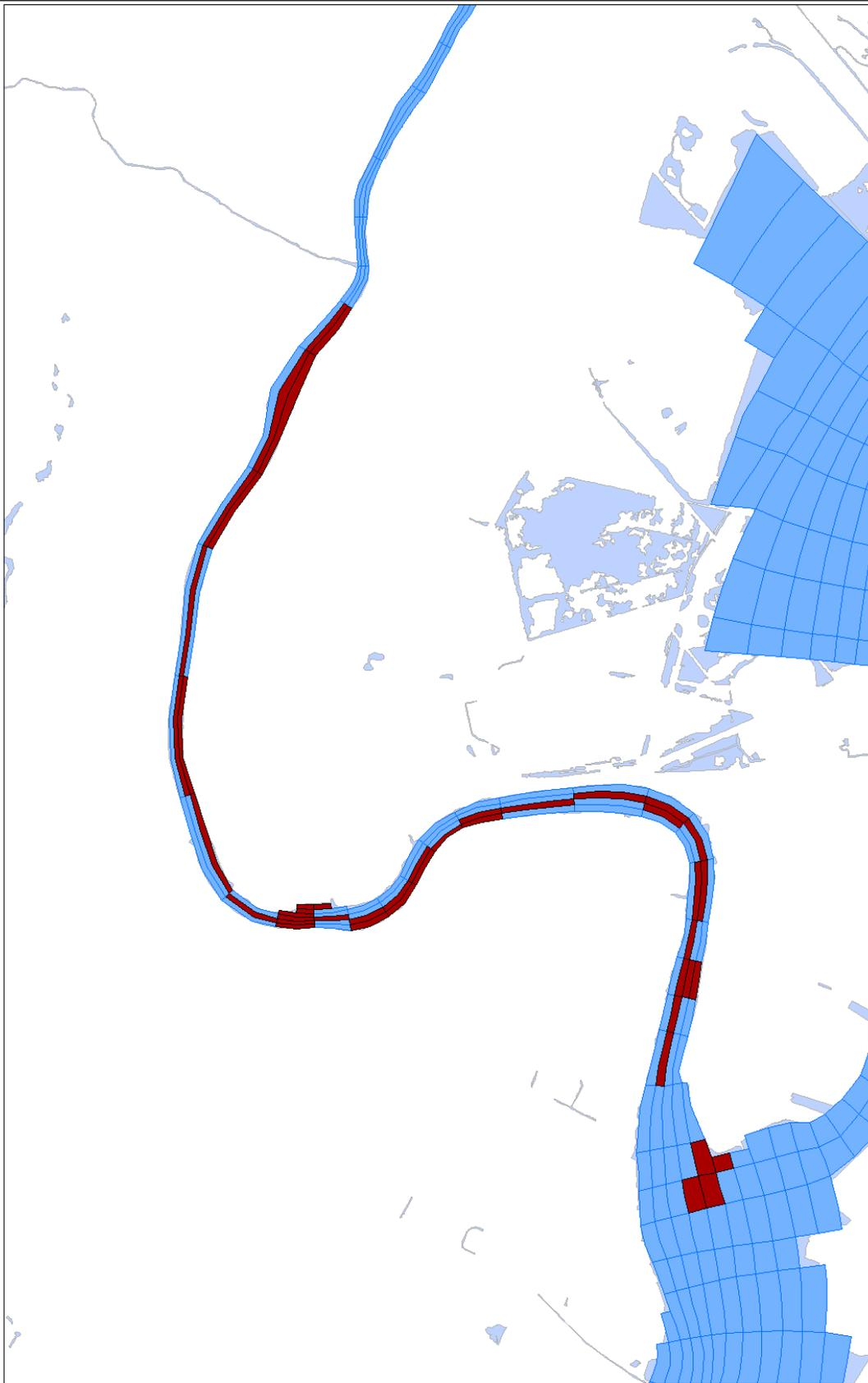
Areas Capped in Alternative 4 - Focused Capping with Dredging for Flooding
