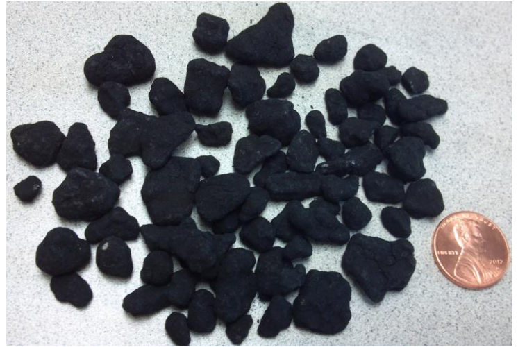
Figure 1. Configuration of PAC-coated particle.
