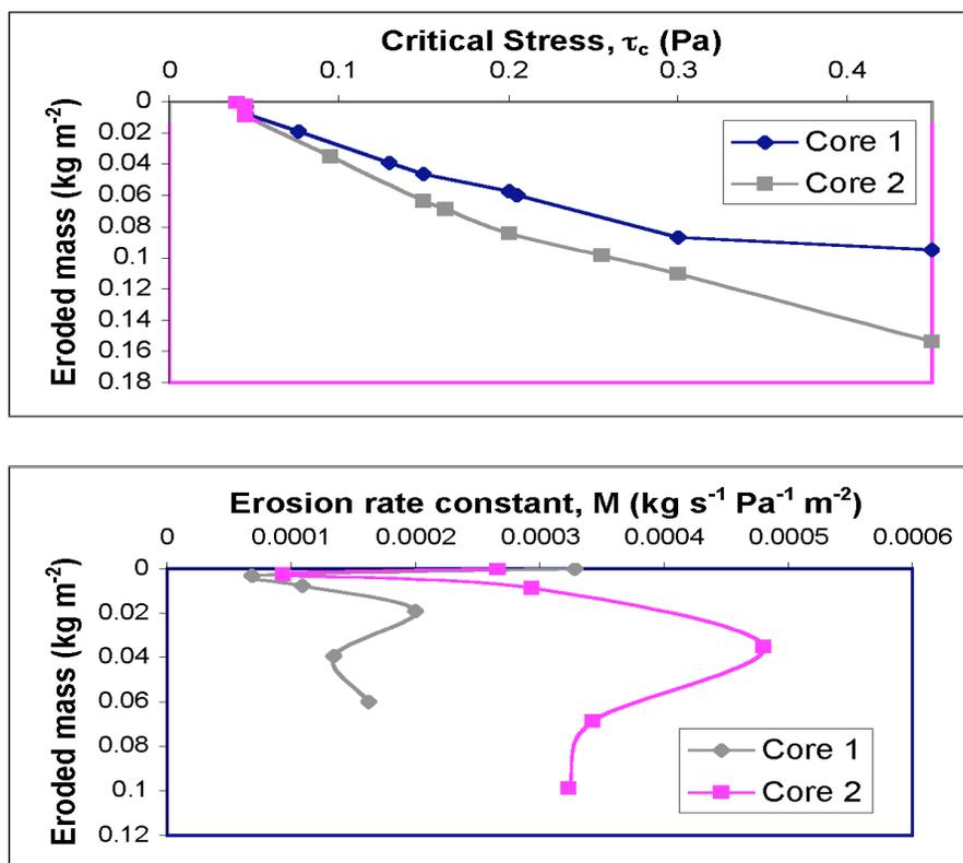
**Figure 3** - Critical stress and erosion rate constant profiles for experiment 1, cores 1 and 2. These cores were collected and eroded on May 16, 2005. The cores were taken in the vicinity of station 9, in a water depth of 2.1 meters. See table 1 and figure 1 for additional information.
