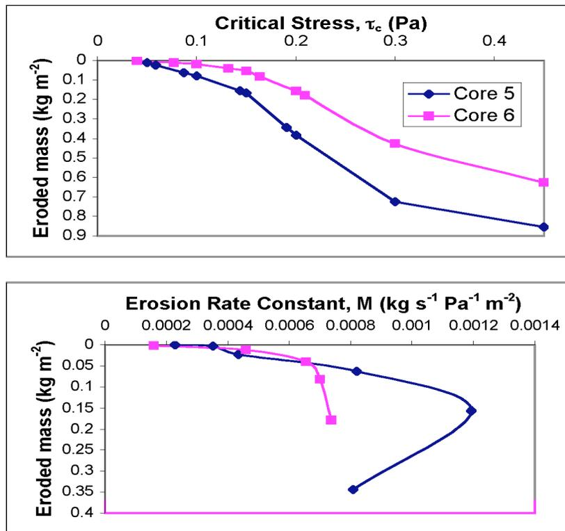
**Figure 5** - Critical stress and erosion rate constant profiles for experiment 3, cores 5 and 6. These cores were collected and eroded on May 17, 2005. The cores were taken in the vicinity of station 1, in a water depth of 8.2 meters. See table 1 and figure 1 for additional information.
