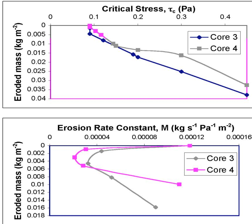
**Figure 4** - Critical stress and erosion rate constant profiles for experiment 2, cores 3 and 4. These cores were collected and eroded on May 17, 2005. The cores were taken in the vicinity of station 13, in a water depth of 1.5 meters. See table 1 and figure 1 for additional information.
