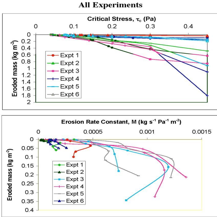
**Figure 2-** Plot of all 12 cores, from 6 experiments, that were tested using the Gust erosion microcosm system from 10 cm cores collected at 6 sites in the Passaic River, NJ. Upper panel shows profiles of critical stress ( $\tau_c$ ) versus eroded mass which is a measure of depth into sediment bed. Lower panel shows erosion rate constant, M, values for all cores. All units are in MKS (meters-kilograms-second) system.
