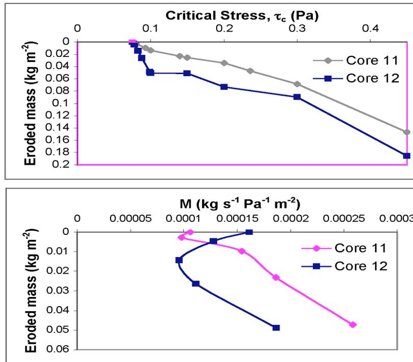
**Figure 8** - Critical stress and erosion rate constant profiles for experiment 6, cores 11 and 12. These cores were collected and eroded on May 19, 2005. The cores were taken in the vicinity of station 5, in a water depth of 1.8 meters. See table 1 and figure 1 for additional information.
