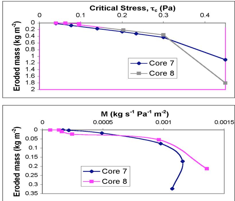
**Figure 6** - Critical stress and erosion rate constant profiles for experiment 4, cores 7 and 8. These cores were collected and eroded on May 18, 2005. The cores were taken in the vicinity of station 3, in a water depth of 2.4 meters. See table 1 and figure 1 for additional information.
