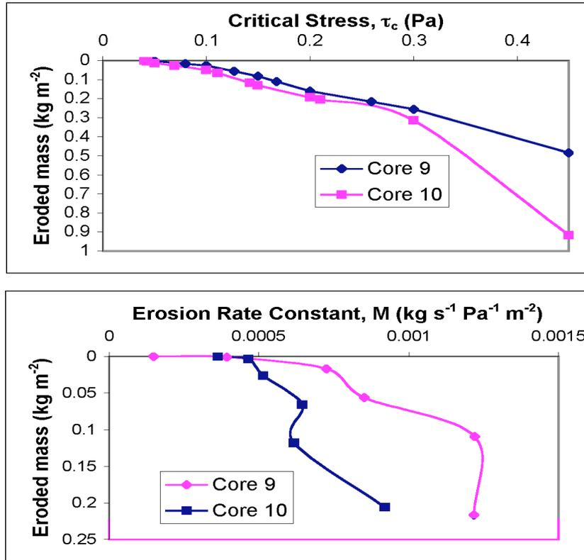
**Figure 7-** Critical stress and erosion rate constant profiles for experiment 5, cores 9 and 10. These cores were collected and eroded on May 19, 2005. The cores were taken in the vicinity of station 6, in a water depth of 3.1 meters. See table 1 and figure 1 for additional information.
